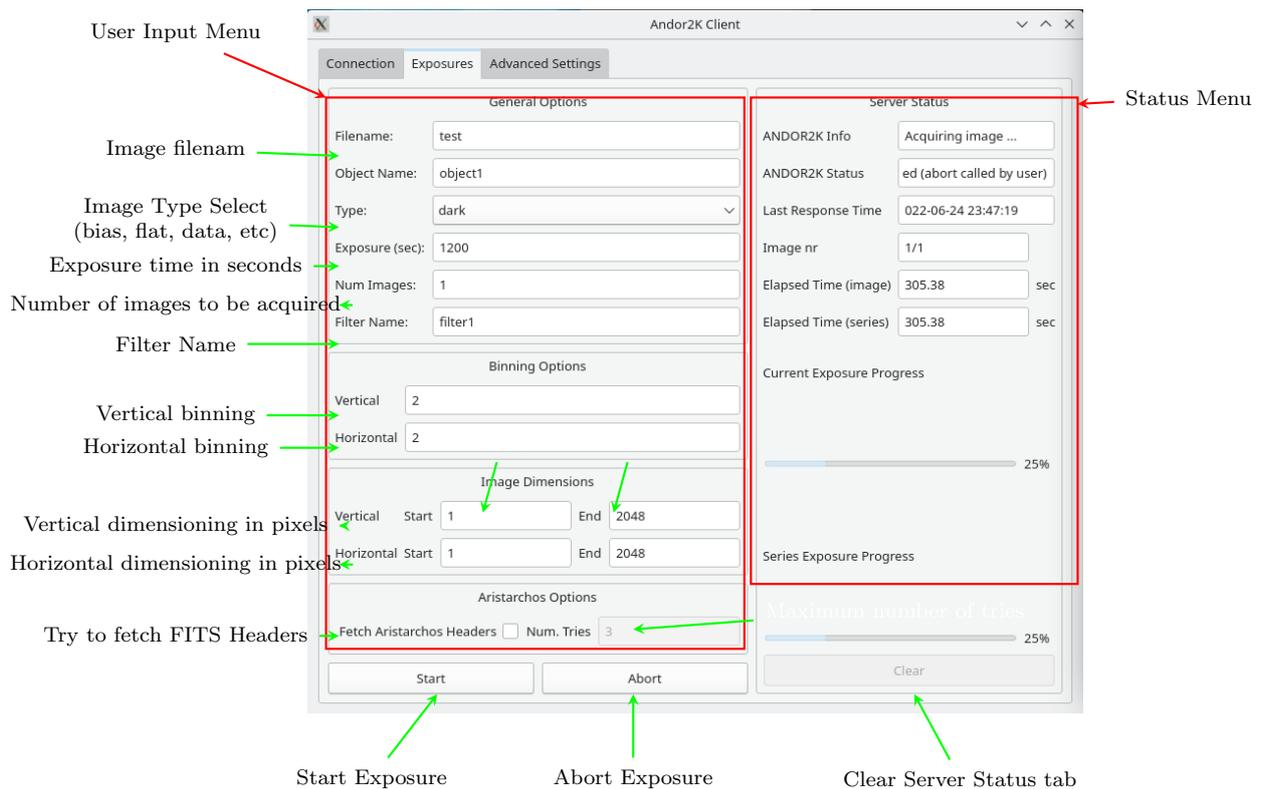
Figure 1.4: andor2k-client detailed view of Exposure Tab
