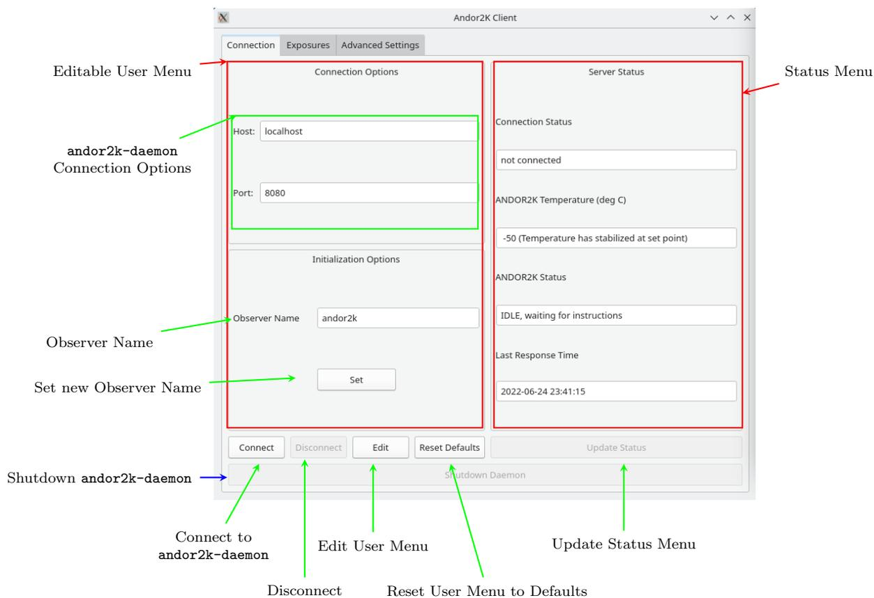
Figure 1.3: Detailed view of `andor2k-client`'s Connection Tab
