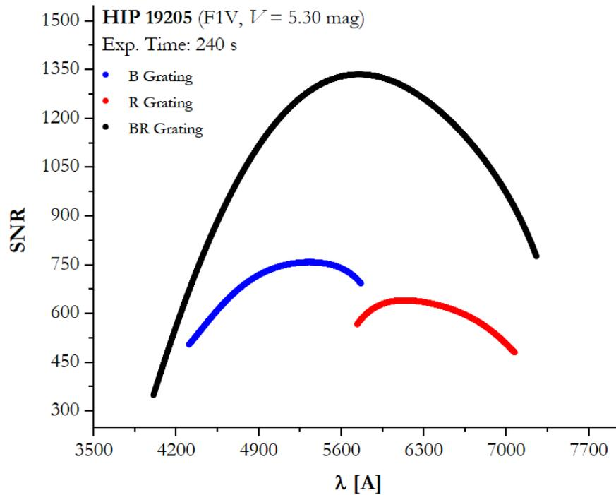
Fig. 30. SNR sensitivity on the spectral range (grating). SNR values are depicted for a A8V (upper), a F1V (lower) spectroscopic standard star.
