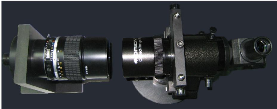
Fig.21. Collimator lens aligned with the small telescope
