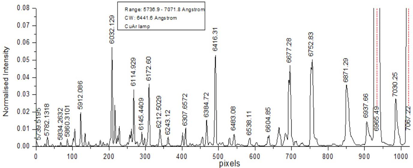
Fig. 23. Arc for the Red 1200 groove/mm grating centered on 6441.6 Å.
