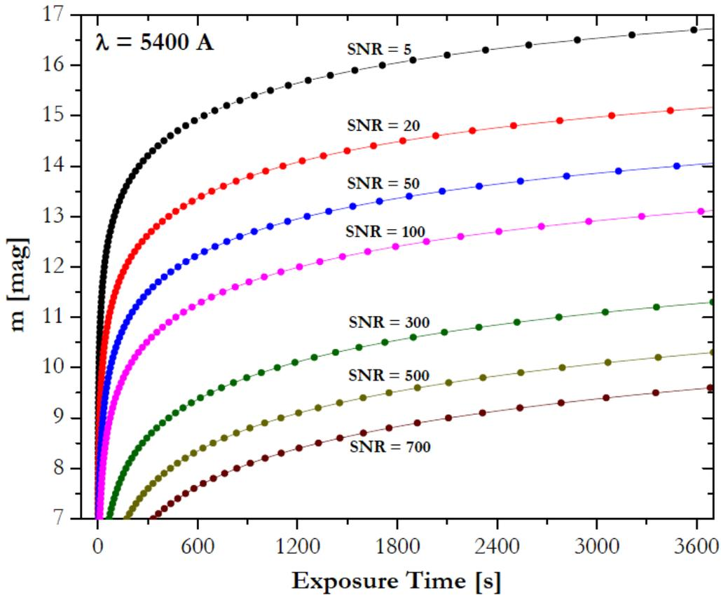
Fig. 34. Magnitude-exposure time curves for a wide SNR range. ATS is inefficient to deal with stars fainter than  $m = 17$  mag.
