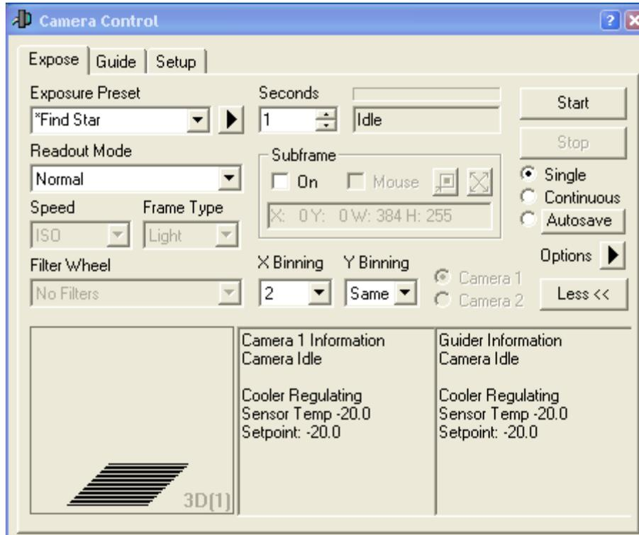
Fig. 13. Expose tab on Camera Control
