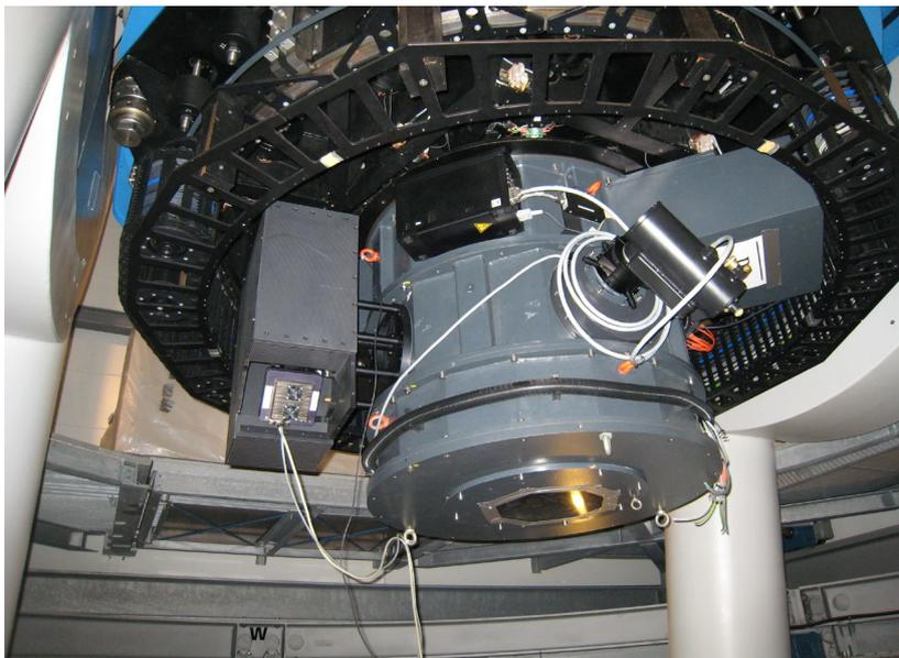
Fig. 1. The ATS spectrometer on the 2.3m Aristarchos telescope
