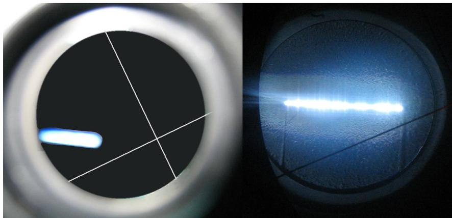
Fig. 22. Fibre image through the eyepiece. Out of focus on the left and focused on the right.
