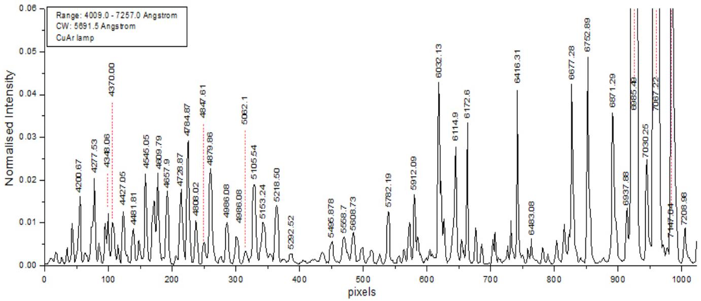
Fig. 25. Arc for the 600 g/mm grating centered on 5691.5 Å.
