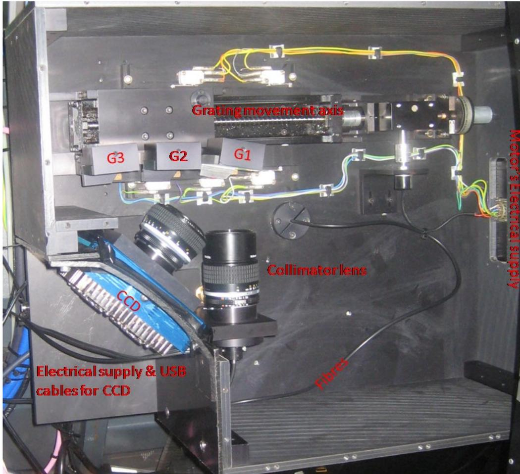
Fig. 3. The mechanical layout of the Aristarchos Transient Spectrometer
