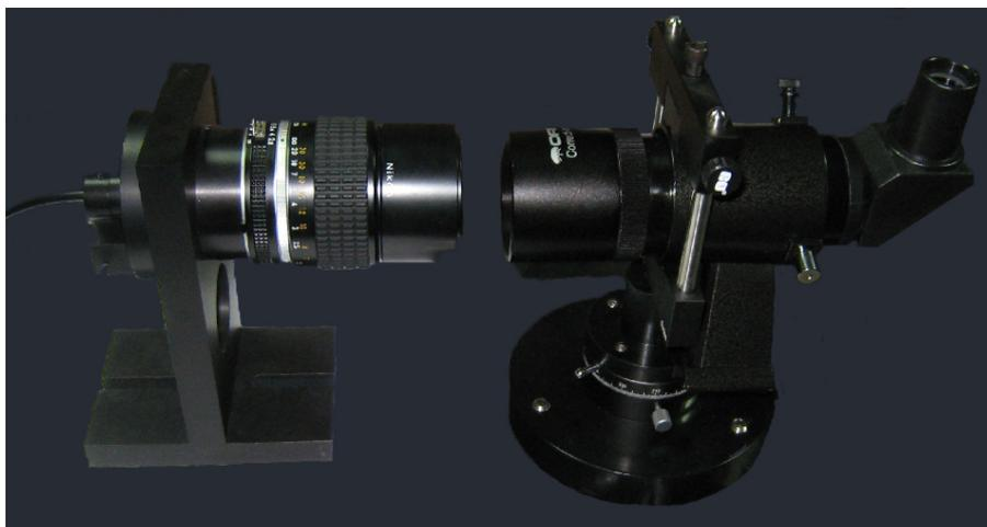
Fig. 19. Collimator lens opposite a small telescope
