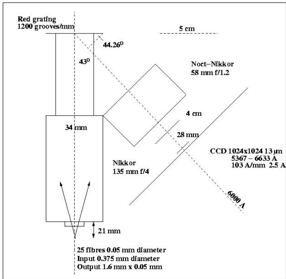
Fig. 2. The optical layout of the Aristarchos Transient Spectrometer (designed by J. Meaburn)
