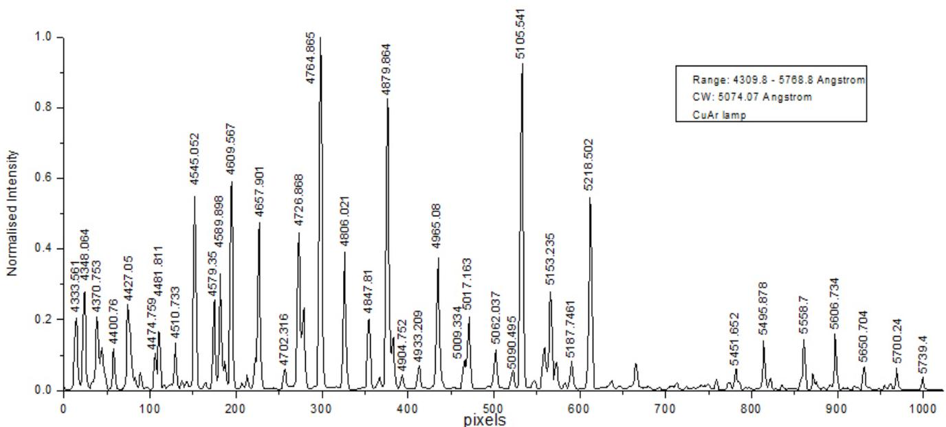
Fig. 24. Arc for the Blue 1200 groove/mm grating centered on 5074.1 Å.
