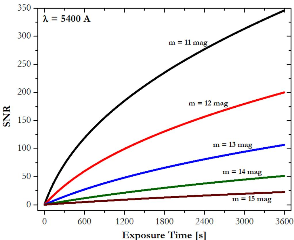
Fig. 33. SNR sensitivity on the brightness and the exposure time. SNR values are depicted for stars lying in the range 11-15 mag and various exposure times less than 1 hr.
