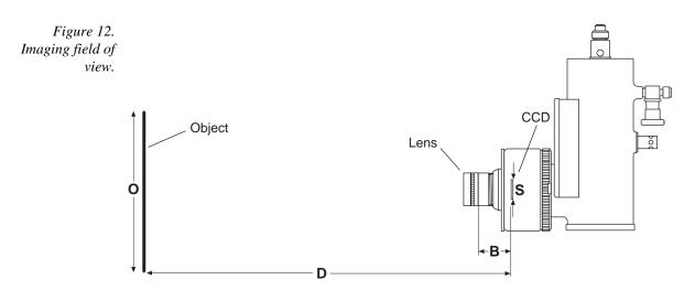
D = distance between the object and the CCD
