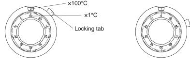
In Figure 10, the knob on the left is set to -90°C. The locking tab is shown in the unlocked position. On the right, the temperature is set to -100°C and the locking tab is in the locked position. Note that the rectangular window reads "1" in this case.
