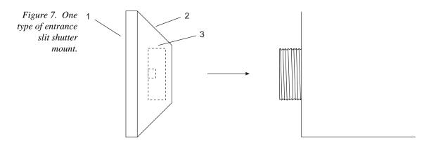
Remove part 1 by removing the four Phillips screws. Place part 2 over the entrance slit, and mount it by threading part 3 to the spectrometer. Replace the shutter and part 1.
