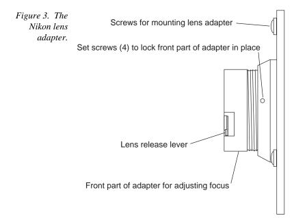
To remove the lens, locate the lens release lever at the front of the lens mount. Press the lever toward the camera housing, and at the same time rotate the lens clockwise. Then pull the lens straight out.
