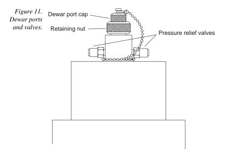
• After the detector has been properly evacuated, loosen the retaining nut (Figure 11) a few turns, then remove the LN dewar port cap by pulling it straight out.
