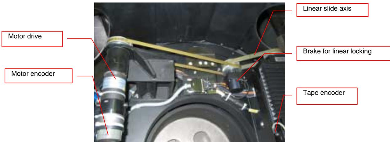
Fig. 5.4\_42. Linear drive system
