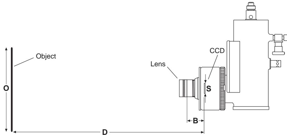
$D$  = distance between the object and the CCD
