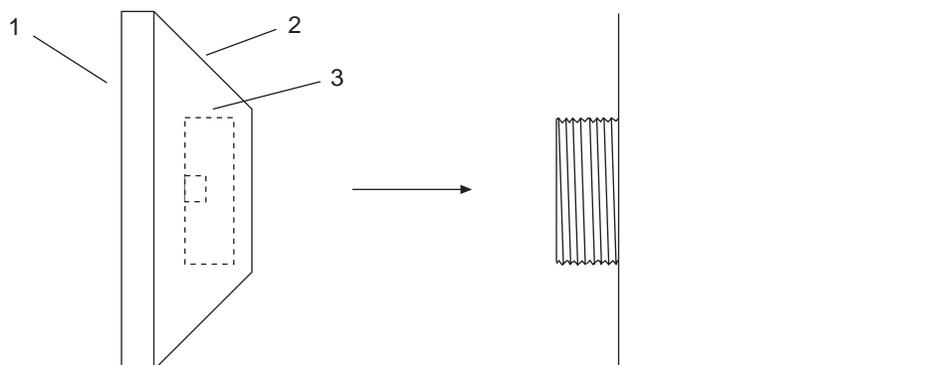
Remove part 1 by removing the four Phillips screws. Place part 2 over the entrance slit, and mount it by threading part 3 to the spectrometer. Replace the shutter and part 1.
