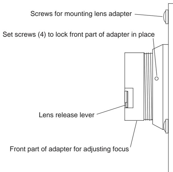
To remove the lens, locate the lens release lever at the front of the lens mount. Press the lever toward the camera housing, and at the same time rotate the lens clockwise. Then pull the lens straight out.
